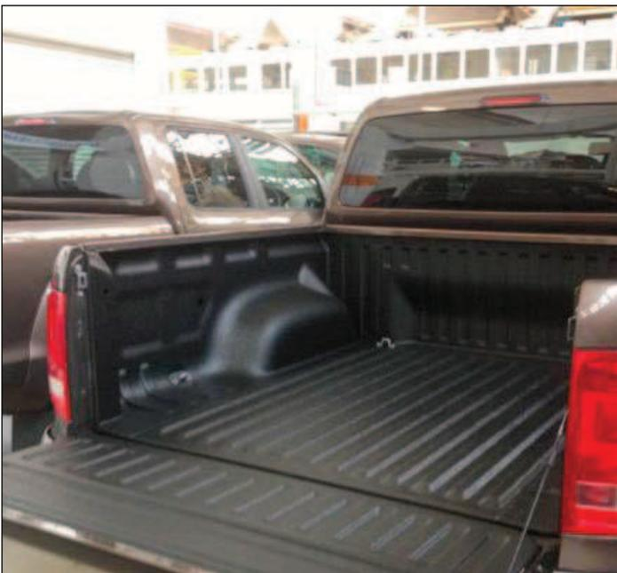
Polyurea is an elastomer created by mixing two reactive components: an isocyanate (the A component) and an amine (the B component). Depending on the desired property profile of the finished coating, additives like pigments, defoaming and fire protection agents are also included.
